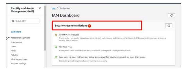
Select the radio button under access key ID, then select action drop-down button then click deactivate. Remember you must first deactivate an access key before deleting it. When prompted proceed and click deactivate.
